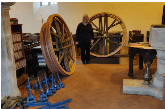
Claire with the refurbished wheels and clappers (photo by Jeanette Davey)
