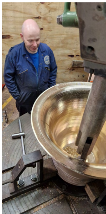
North Moreton's new bells: left: at the Eijsbouts Foundry and right: being tuned at Whites of Appleton.
